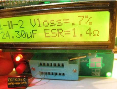
These CHC BRANDED CAPACITORS ABOVE PICTURED.. (they have "low esr"wording on the capacitor) were measured on average to be 1.0 to 1.1 ohm and one of them measured 1.4 ohms.
